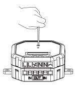
To set the device into pairing mode use the pin to press the button for 2 seconds. The device will then go into pairing mode.
