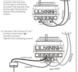
5. Wall installation Remove the existing wall switch. This receiver is a replacement for the existing wall switch and it is not suitable if the existing light switch is interconnected to the other light switches for multi way switching. Do not exceed the maximum load: 300W. 6. Connect the live wire and the switch wire: Connect the live wire to the [L] contact. Connect the switch wire to the [x] contact.
