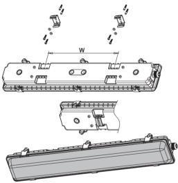
4. Remove the lamp board, as shown below.
