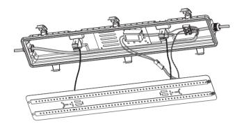
6. Assemble the lamp board back to the lamp.
