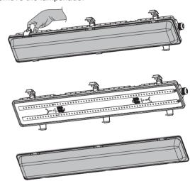
5. Disassemble the waterproof fixed-head at first, and reassemble after power line is installed.
